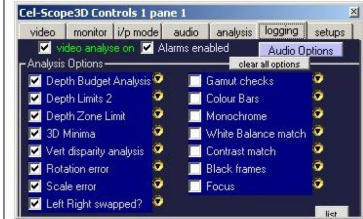
Each test parameter can be individually selected and setup according to its own parameter menu. All disparity settings can either be in pixels or screen percentage.
