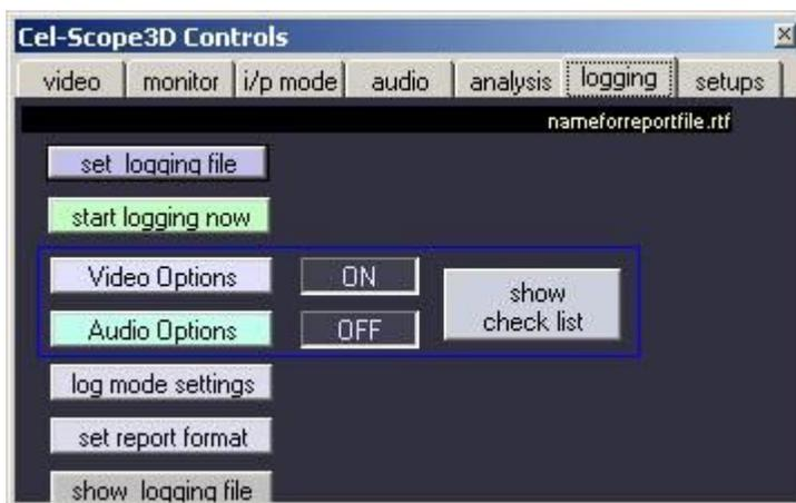
The logging menu is used to set the file destination and formatting styles and options. A pre-flight check list ensures no ambiguity on what is about to be run
